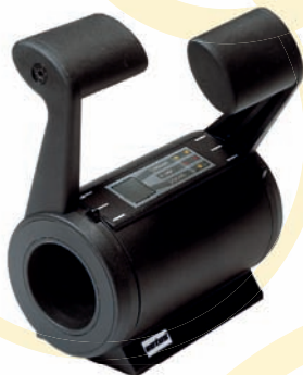
Single lever control handle for two engines (Throttle and gearshift) (2)
