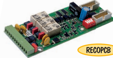
Interface card for auto-synchronisation of two engines. (6)
